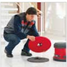
A pad and steel wool ring are required for spray crystallisation of marble floors.
