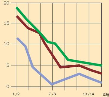
The oxygen content clearly demonstrates the difference between the various bin types. The pH-value inside the non-ventilated bin is 5.0 and inside the Compostainer® it is over 7.0.
