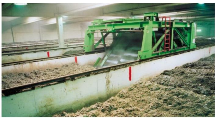
The Biofix system processes biodegradable waste in an automated and dynamic process to recycle it into a high-quality compost or produce landfill material complying with the legal requirements, laid down in the various directives.
