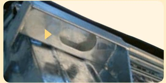
**Chip nest** on the underside of the comb lift bar for fitting an identification chip
